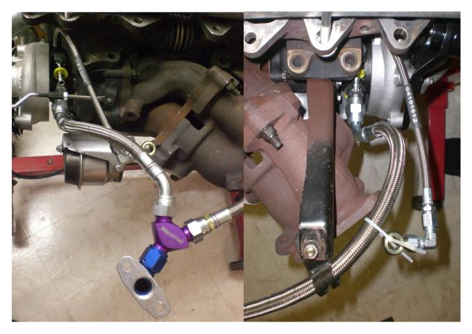
The picture on the Right is the #2 Turbo oil drain line. It has a 90 degree on the turbo side and a straight on the other. Notice how the stock hose "C" Clamp is holding the hose in place. The small hose to the right is the oil inlet for the #2 turbo.
