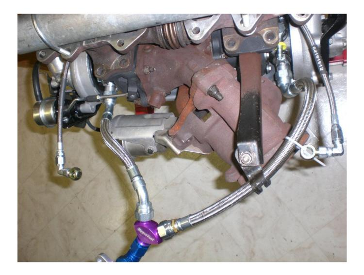
This is the overall view of both the -10AN Return lines and the two -4AN Oil inlet lines. The two oil inlets bolt to the block with the stock 12mm banjo bolt. The kit includes 4 new Toyota crush washers.
