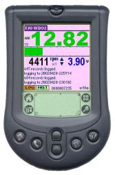
The datalogging and analysis software provides the functionality to display, log, and analyze the data from the wideband controller. AFR plots can be viewed in real time, playback, or on static
