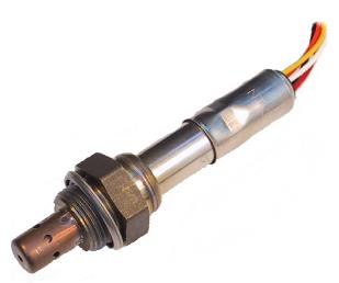
exhaust stream) is **lower** than the body (the part where the wires exit). The mounting position should be chosen such that the sensor will never become submerged. Tighten the sensor to 45 N-m [33 lbf-ft]. Over tightening or cross threading during installation will cause irreparable damage to the sensor – if the sensor does not thread in easily and smoothly DO NOT FORCE IT – check the threads as they may need to be cleaned or re-tapped.
