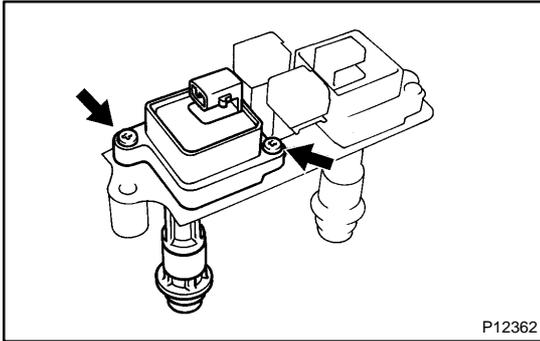
5. REMOVE IGNITION COILS FROM BRACKET
