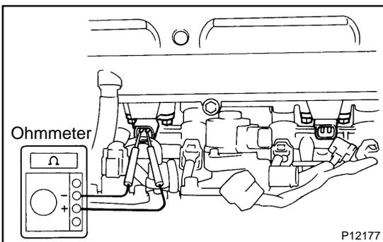
**4. INSPECT CAMSHAFT POSITION SENSORS**
